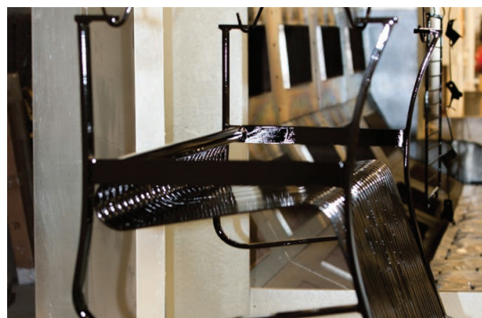
Curing Powder Coat
